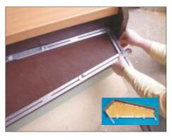
With the angle template you can forms, like a stair, transfer very easy and fast.
