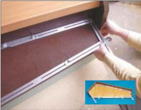
With the angle template you can forms, like a stair, transfer very easy and fast.
