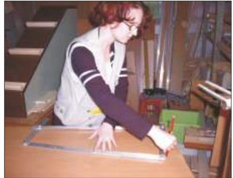
With the angle template you can easily transfer the form to the new board or a paper template.
